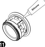
Apply a generous amount of 100% silicone to underside of WingTite drain flange.
