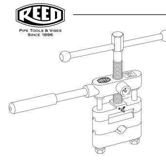
CSO1 <sup>3</sup>/<sub>4</sub>" - 1" (19-25 mm) CSO2 1 <sup>1</sup>/<sub>4</sub>" - 2" (32-51 mm) **Shutting off flow:** Assemble tool handle where desired. Unscrew the main feed screw. Lift and swing out dies to allow tube to seat between crimping dies. Swing dies back over the tie rods. Turn the feed screw to compress the tube using only enough pressure to shut off flow.
