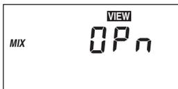
The control is no longer able to read the mixing supply sensor due to an open circuit. In this case the control will operate the injection pump at a fixed output as long as there is a mixing demand. Locate and repair the problem as described in the Data Brochure D 070. To clear the error message from the control after the sensor has been repaired, press the **Item** button.
