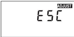
To exit the ADJUST menu, press and release the **Item** button to advance to the ESC item. Then either press the ▲ or ▼ button, or leave the buttons alone for 20 seconds.
