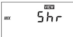
The control is no longer able to read the mixing supply sensor due to a short circuit. In this case the control will operate the mixing valve at a fixed output as long as there is a mixing demand. Locate and repair the problem as described in the Data Brochure D 070. To clear the error message from the control after the sensor has been repaired, press the **Item** button.
