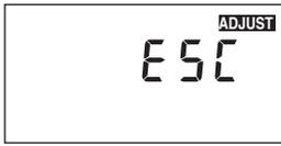
To exit the ADJUST menu, press and release the **Item** button to advance to the ESC item. Then either press the ▲ or ▼ button, or leave the buttons alone for 20 seconds.
