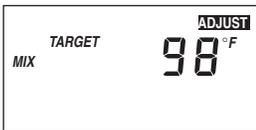
Press and release the **Item** button to advance to the MIX TARGET adjustment. Use the ▲ or ▼ button to select the desired temperature. The MIX TARGET setting is set to the desired setpoint supply temperature.
