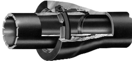
The AMERICAN Flex-Ring Joint provides flexible joint restraint against thrust due to internal water working pressure or external forces. It is also used in horizontal directional drilling (HDD) and pipe bursting applications.
