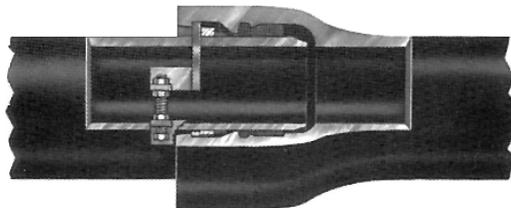
The AMERICAN Lok-Ring Joint is furnished in sizes 54"-64" and provides flexible joint restraint against thrust due to internal water working pressure.
