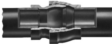
The AMERICAN Flex-Lok Joint, furnished in sizes 30"-60", is a boltless, very flexible joint. This joint is designed to provide up to 15° joint deflection for subaqueous or other difficult installations. Contact AMERICAN for 64" size requirements.
