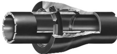
The AMERICAN Field Flex-Ring provides dependable and flexible field-adaptable restraint against thrust due to external forces or internal water working pressure in the standard Flex-Ring joint. This joining structure is also recommended at locations where field cutting is required in 14"-36" Flex-Ring piping.
