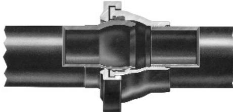
The AMERICAN Flex-Lok Joint, furnished in sizes 4"-24", is a boltless, very flexible joint. This joint is designed to provide up to 15° joint deflection for subaqueous or other difficult installations.
