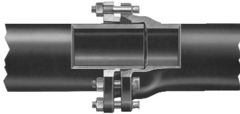
The AMERICAN Mechanical Joint, furnished in pipe sizes 4"-12" and in fittings sizes 4"-48", is a flexible stuffing box type connection used primarily in underground service.
