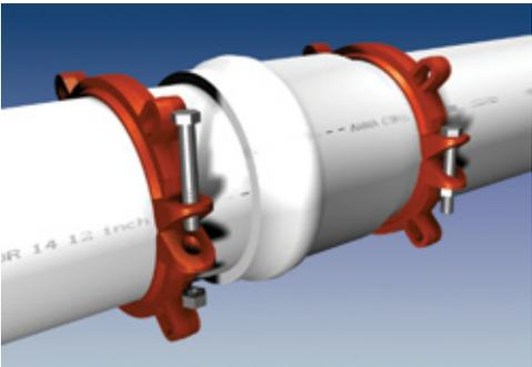
5. Install both halves of the restraint ring at the proper location, tapping each half into place. Make sure that the complete ID of the ring is touching the pipe before installing the side bolts. Tighten the side bolts evenly to 110 ft-lbs. (60 ft-lbs on 4" and 6")
