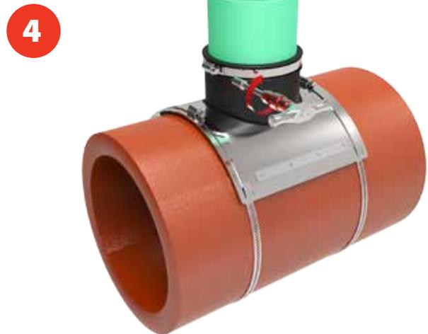
Loosen lateral inlet worm drive clamp. Insert lateral pipe into mouth of inlet until it rests against the internal pipe stop. Tighten lateral inlet worm drive clamp to 60 in/lbs. of torque.
