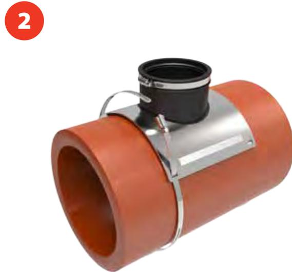
Core appropriate sized hole into sewer main (4" core i.d. of 4.60" - 4.90" & 6" core i.d. of 6.60" - 6.90"). After making sure pipe surface is clean and free of debris, wrap stainless steel apron and gasket around sewer main, making sure internal flange of gasket is centered in hole of cored pipe.
