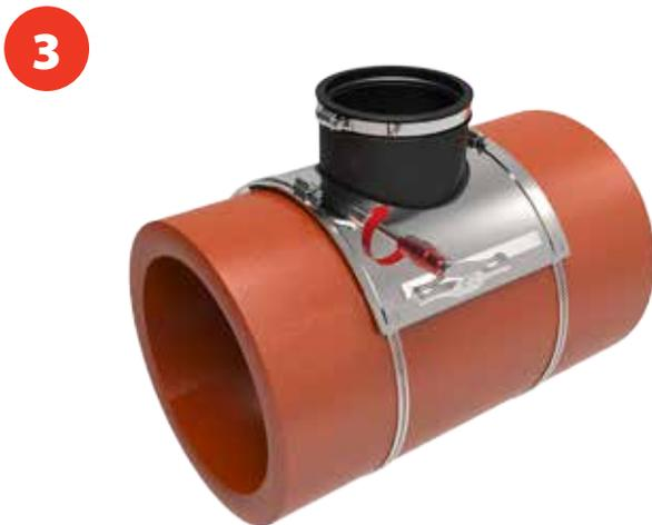
Pull screw head away from clamp housing and pull "tail" through housing. Cinch down clamp to hand-tight. Note: Housing should be centered onto apron. Repeat clamp installation on opposite side. Using a nut driver or torque wrench, tighten quick-release clamps alternately and firmly to 60 in/lbs. of torque. Slide clamp "tail" back through top of square eyelet.
