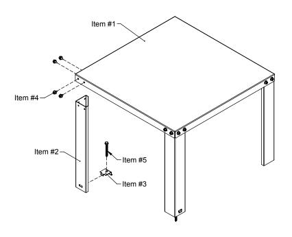
The QUICKSTAND™ #40-S-22- (A or U) stands safely elevates water heaters and other equipment above the floor (650 lbs rating).
