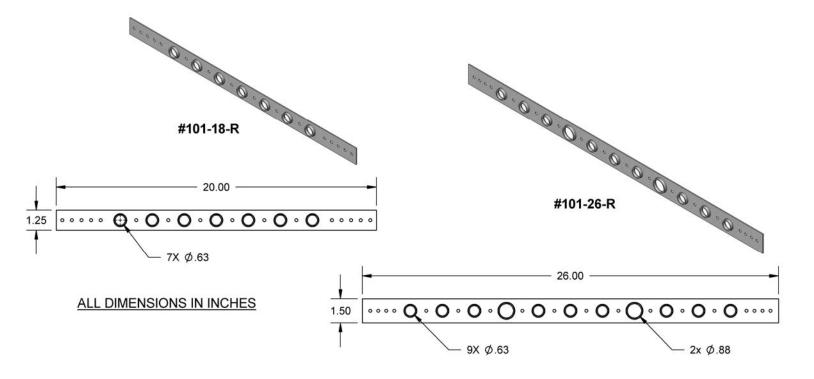
The HOLDRITE<sup>®</sup> #101-18-R and #101-26-R are Copper-Bonded<sup>™</sup> steel brackets with extruded holes. The #101-18-R has 5/8" holes on 2" centers. The #101-26-R has 5/8" holes on 2" centers and 2 - 7/8" holes on 8" centers. Each to support ½" or ¾" copper tubing. The #101-18-R and #101-26-R position copper water supplies for sinks, water closets, and other fixtures. When soldering, heat the pipe, not the bracket.
