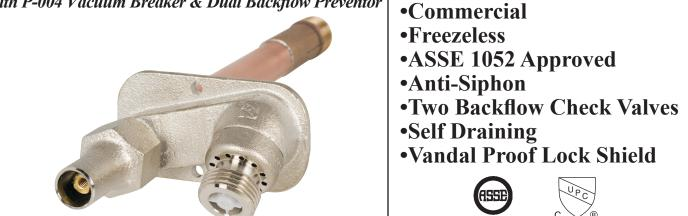
The PRIER C-534 provides a year round source of water to areas of structures that are subject to freezing temperatures. The hydrant valve is connected to the supply piping in the heated portion of the structure, eliminating the possibility of freezing. To assure freeze protection, the hydrant will drain even with the hose attached and under pressure without sprayback!
