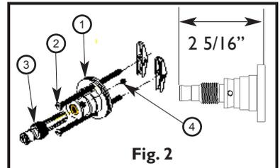
4. Engage POST (3) into FLANGE (1). Position POST (3) height to 2 5/16" from mounting surface. Secure POST (3) into place by tightening SETSCREW (4). See Fig. 2.
