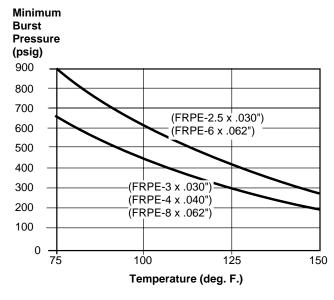
Suggested working pressure of polyethylene is 1/3 of burst pressure at system operating temperature.
