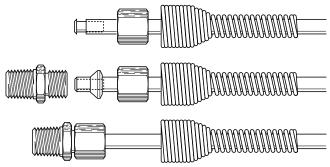
2. Install nut on hose, insert brass tube support.
