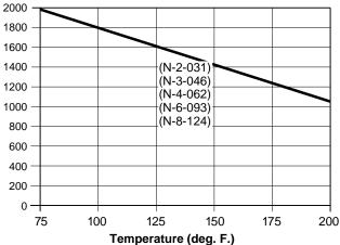
Suggested working pressures are 1/4 of burst pressure at system operating temperature.
