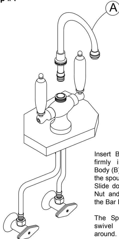
Insert Bar Spout (A) firmly into the Bar Body (B), making sure the spout bottoms out. Slide down the Spout Nut and tighten it to the Bar Body.
