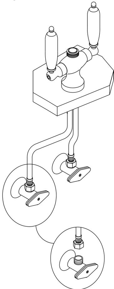
Attach the Hot and Cold Supply Hoses to the angle supply valves (Not supplied).
