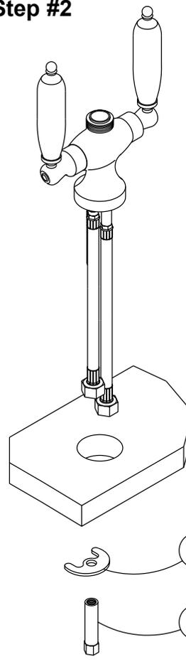
Position the Bar Body over the mounting hole as shown. (Note: The Handles pull forward to turn on.) The Mounting Bracket must be in the back.) Feed the Bar Supply Hoses (C) through the mounting hole on the counter.
