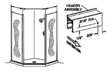
Press the header assembly [D] over the wall jambs [E] and 135° posts [K]. Check the posts for plumb. Adjust as required by varying the overlap of the header over the wall jambs. You may need to trim the ends of the header where it meets the wall. The minimum horizontal dimension for the door opening is the door panel width (see the graphic in Step #9) plus 1/2", maximum is the door panel width plus 1 3/4".
