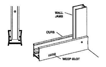
Wipe the shower walls and sill, curb assembly [A] and wall jambs [E] with a clean, dry cloth to remove any dust or debris. Apply a 1/4" bead of caulk along the inside of both of the pencil lines marked in Step #3. Carefully replace the curb in the exact position marked. Caulk the inside of the curb ends where they meet the wall. Caulk around the anchor plates [B], screws [C], and the insides of the mitered joints.
