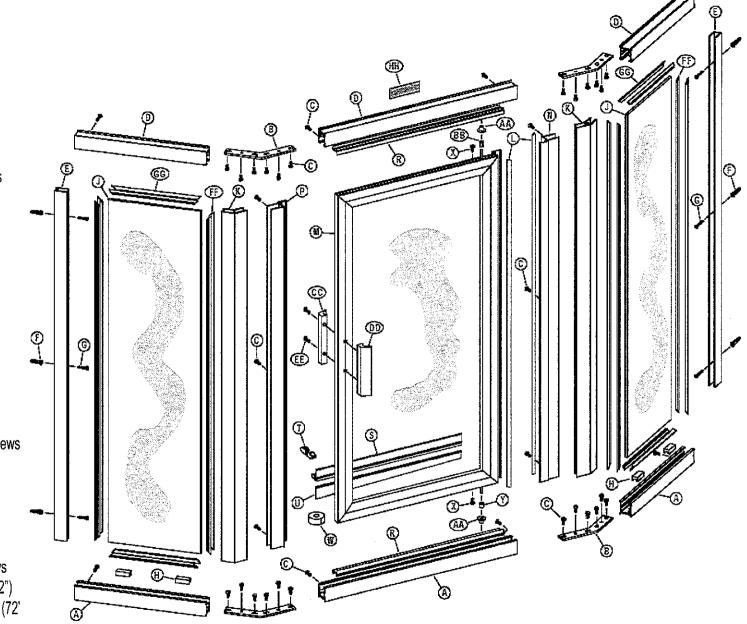
The BASCO 160/760 Thin-Line Shower Enclosure is completely reversible and may be installed pivot-left or pivot-right. For maximum waterproofing, the pivot jamb should be opposite the shower head. Use the diagram to determine the correct position for the door in your particular Thin-Line installation. This instruction sheet depicts a pivot-right installation.
