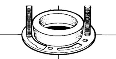
**Alternate way is to place wax ring on the “horn” of the bowl (bowl shown upside down).**
