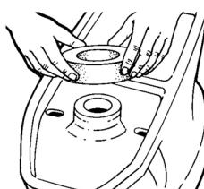
**D****STRADDLE BOWL, LIFT INTO PLACE THEN SET STRAIGHT DOWN ONTO RING AND BOLTS.**
