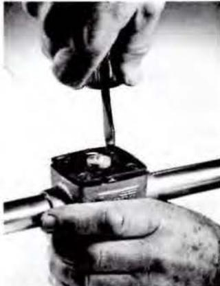
2—Remove the 4 Screws from hold down plate
