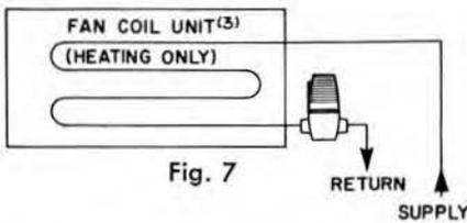
(3) May also be used for cooling if by-pass is provided in piping to prevent chiller freeze-up.
