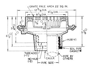
CONFORMS WITH ASTM-C564.
