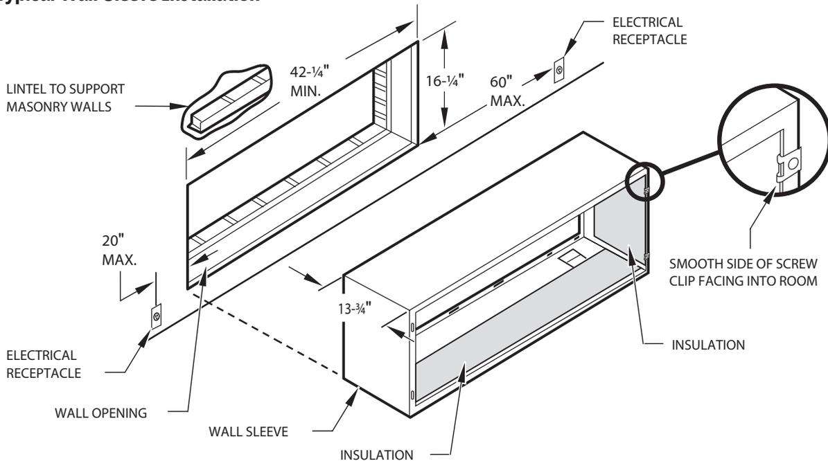
**NOTE:** All 230/208V units are manufactured with a 60" power cord and all 265V units with a 18" power cord.
