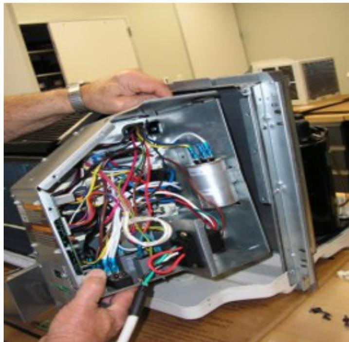
Figure 417 (Removal of Control Compartment)
