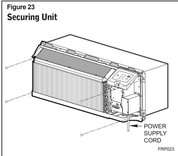
2. Locate the four supplied chassis mounting screws. Insert the screws through the chassis mounting flange holes that are aligned with the speed nuts in the wall sleeve. Tighten all four screws (two per side).
