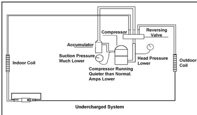
Figure 601 (Undercharged System)
