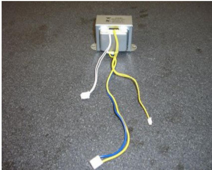
Figure 421 (Transformer Removed)
