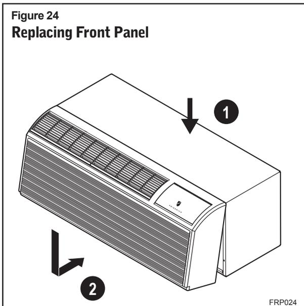
3. Place tabs over top rail (1). Push inward at bottom until panel snaps into place (2).
