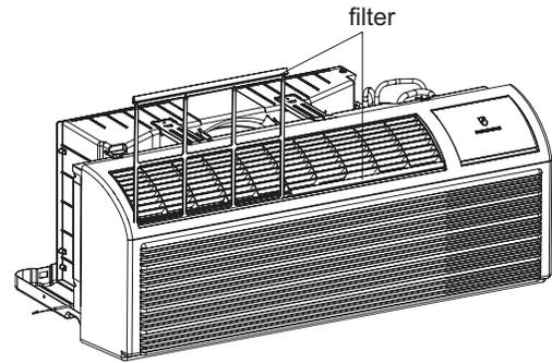
b Drag the lower part of panel, pull it outwards and upwards to left separate from clasps, and then remove the front panel.
