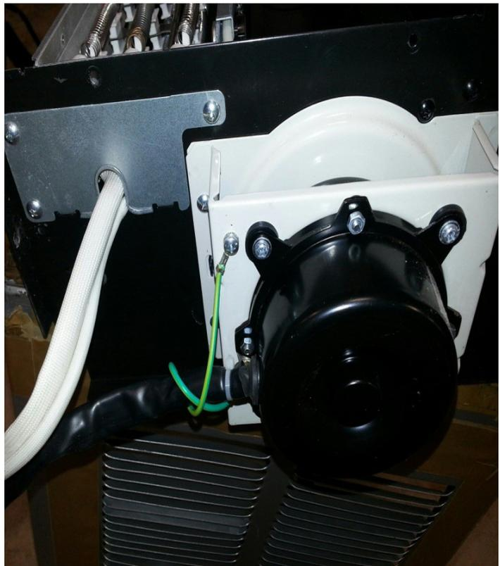
**Figure 407 (Remove Housing, Indoor Motor and Heater)**
