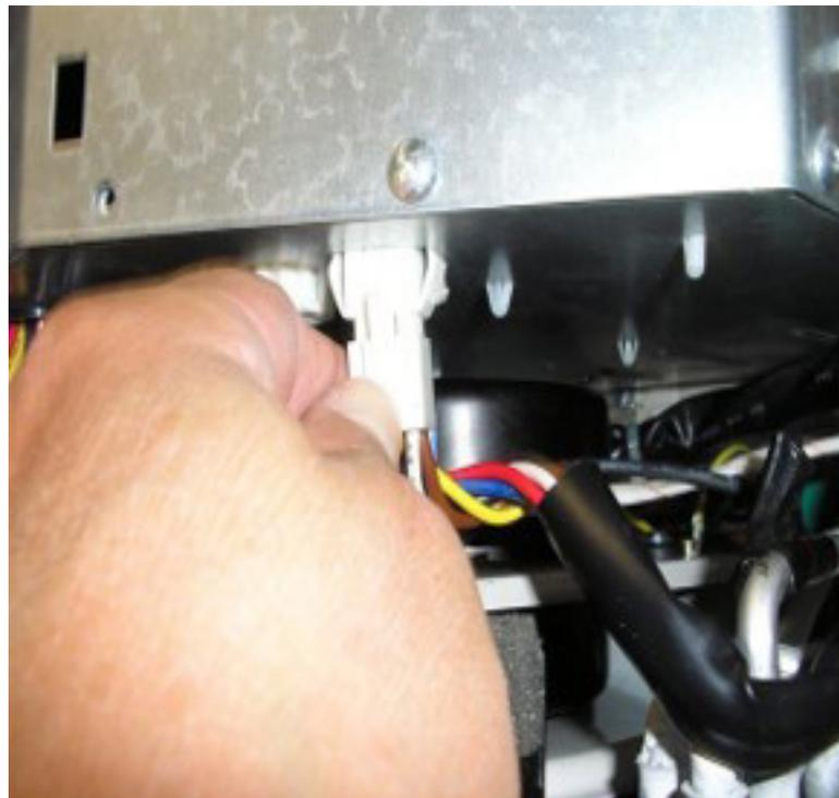
**Figure 416 (Power Cord, Indoor Motor, and Heater Connections)**
