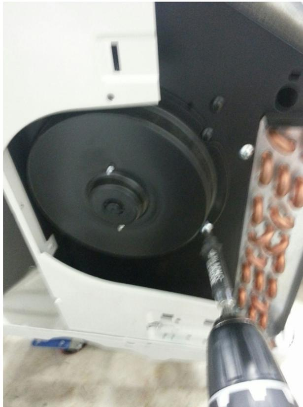
**FIGURE 403 (Removal of Indoor Fan Grommet)**
