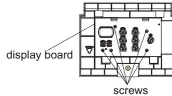
c Remove 4 screws fixing baffle plate of electric box and then remove the baffle plate of electric box.
