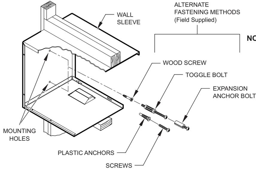
**NOTE:** The Wall Sleeve must be horizontally level (side-to-side) and pitched 1/4 bubble to the outside when installed in an opening. The mounting hole location should be approximately 2-4" from the top and bottom of the sleeve.
