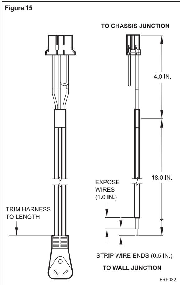
3. Route the cut ends of harness through the conduit connector assembly and flex conduit sleeve. Be sure to use the supplied conduit bushing to prevent damage to the cord by the conduit.
