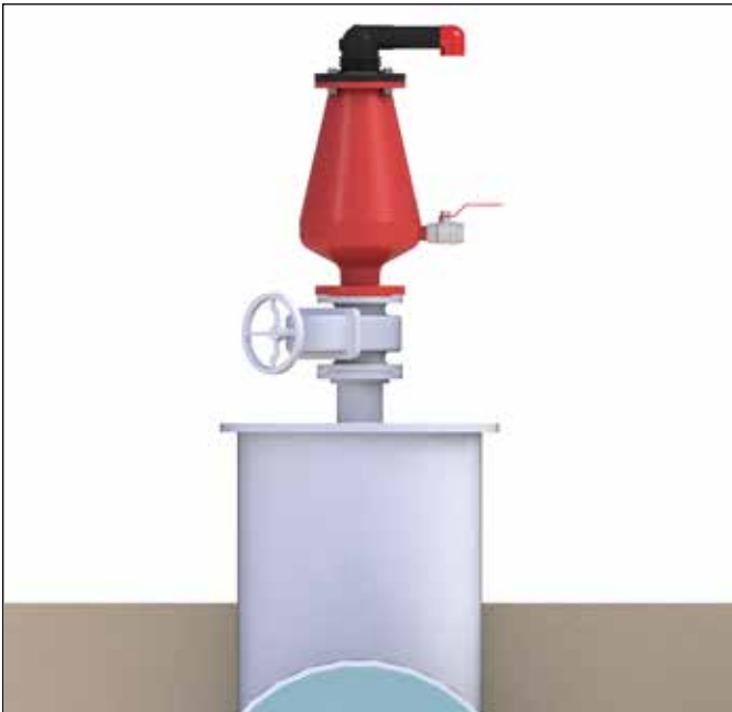
Single Air Valve on an Isolating Valve at 45° to Air Valve outlet
