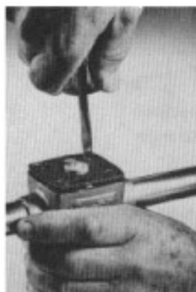
Remove the 4 Screws from top down plate
