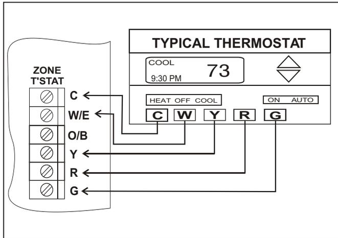
Figure 2b. Typical Hard Wired Heat/Cool type thermostat wiring on any zone.
