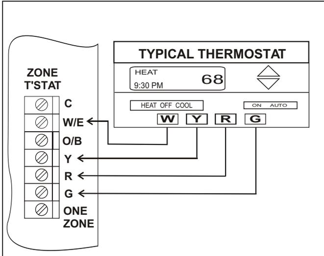
Figure 2a. Typical Battery or Power Robbing type Heat/Cool thermostat wiring on any zone.
