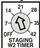
The W2 TIMER sets the total amount of time delay before second stage heating is energized. 1st stage heat will stay energized when 2nd stage heat activates. If desired turn the Timer OFF and let your heat pump thermostats stage up for you.
