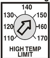
The Heating Limit potentiometer sets the supply air temperature at which the heating is cycled off and the fan continues to run until, the supply air temperature has dropped below the heating limit set point. 3 Minutes min.
