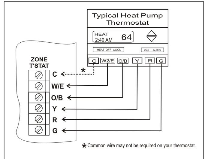
Figure 2d. Typical Heat Pump thermostat wiring on any zone. Note that your thermostat may not have a common wire connection.
