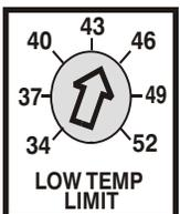
The Cooling Limit potentiometer sets the supply air temperature at which the cooling is cycled off and the fan continues to run until, the supply air temperature has risen above the cooling limit set point. 3 Minutes min.
