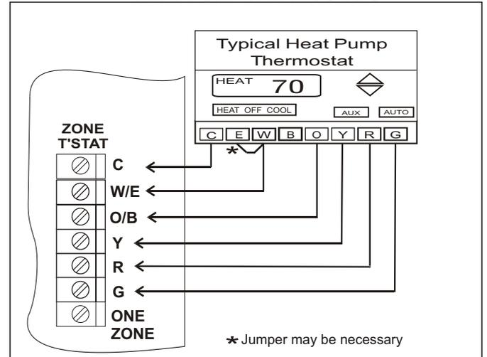
Figure 2c. The NCM300 will accept heat pump style thermostats in all zones. This allows you to energize 2nd stage heat thermostatically instead of through the W2 timer. Also, Emergency heat can be activated from any zone.
