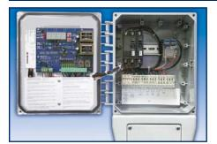
EZ Series® control panels **combine circuit board technology and easy operation** for single phase **simplex**, **duplex and plugger** applications. Each panel features a NEMA 4X enclosure with lockable latch, red LED alarm beacon, audible alarm and more. An **optional mounting post** featuring a **removable access door** for easy wiring is available. For a complete list of models and options available, visit **www.sjerhombus.com**.
