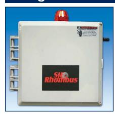
This panel provides a reliable means of controlling one single phase pump in water and sewage installations. Two control switches activate a magnetic motor contactor to turn the pump on and off. If an alarm condition occurs, an additional alarm switch activates the audio/visual alarm. Approved for Halifax, Edgecombe, Warren, Wilson, Cleveland and Brunswick\* counties.
