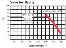
WARNING:T/S-100-NE valves are designed for temperatures up to 366°F, utilizing low presure steam at 150 WSP MAXIMUM
