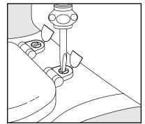
Use a screwdriver to tighten bolt.
