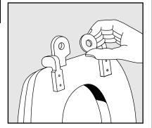
Attach washer to bottom of hinge.
