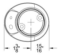
3. The hole in the Monitor Housing should be centered on the mounting hole. If cutting or drilling a mounting hole, please note that the Monitor Housing is elliptical and the hole which runs through it is off center from front to back.
