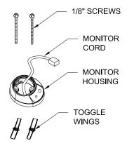
4. Feed the Monitor Cord through the 1 <sup>1</sup>/<sub>4</sub>"diameter Monitor Housing opening so that it is positioned above the Monitor Housing.
