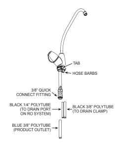
6. Connect the tubing to the Faucet. Push the Blue 3/8" Polytube into the 3/8" Quick Connect Fitting. Push the Black 3/8" Polytube onto the large Hose Barb. Push the Black 1/4" Polytube onto the small Hose Barb.
