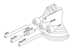
Locate the ¼" Red Feed Water Tubing. Remove the red plug from the fitting labeled "In" on the manifold and insert the tubing. Reference the special supplement sheet in the carton for proper connection of all tubing and removal of plugs. Run the tubing along its course to the Feed Water Saddle Valve, trim to length. (Refer to Fig. 1).
