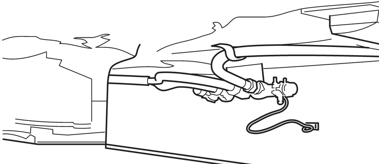
5. If a manifold is used, it shall be rigidly mounted to the I-beam flange. This applies to parallel system layouts. Gas pressure in HUD Code homes is limited to 14 inches water column maximum. Line pressure regulators are not necessary for this pressure and should not be used.
