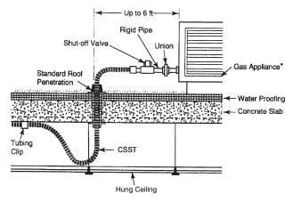
Figure: 4-16 Short (1-6 foot) outdoor connection to roof mounted equipment
