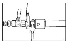
9. Thread nut onto adapter previously installed on the equipment. Using appropriate wrenches, hold adapter and tighten nut to proper torque specified. Do not over tighten or use any pipe dope or thread sealants on this connection. This is a metal-to-metal seat and will not seal if pipe dope or thread sealants are used. Sealants are to be used on the NPT connection to the equipment only!
