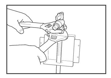
Thread 90 degree ball valve onto nut and tighten so valve outlet faces forward. It is recommended that crescent wrenches be used to avoid damaging valve or nut.
