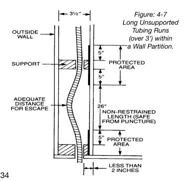
b. At support points and points of penetration 2 to 3 inches from any edge of stud, joist plate, etc. shielding is required throughout area of support. Use a quarter striker plate in these locations. (Figure: 4-8).
