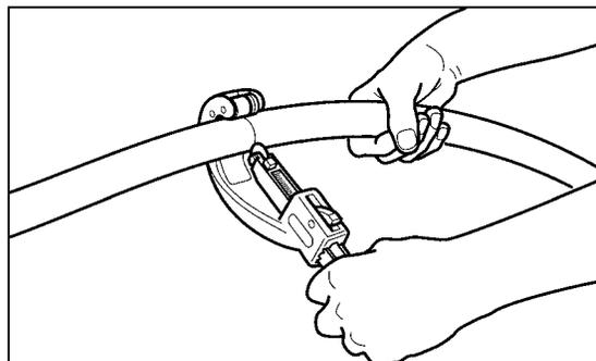
1. Unreel pipe into trench or on the ground and cut to desired length plus one additional foot. Cutting up to 1" size can be done with a large tubing cutter. For 1-1/4 to 2 inch sizes, a reciprocating saw is recommended.
