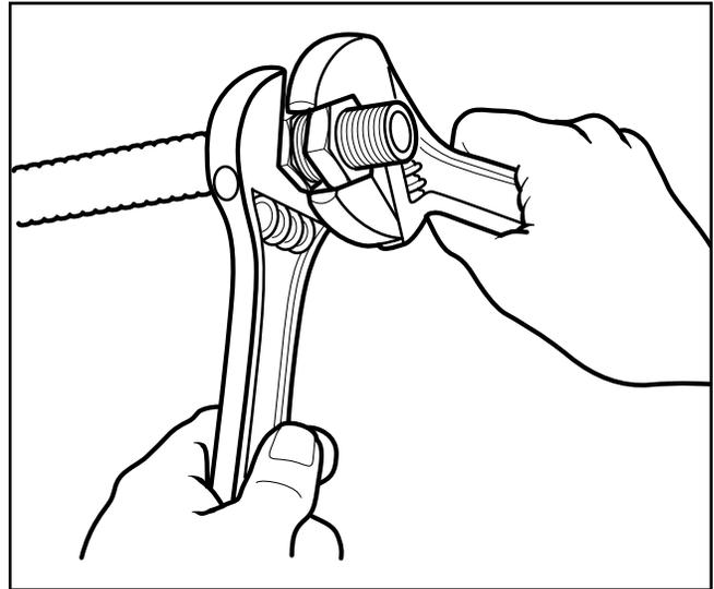
5. **FINAL TORQUE:** Tighten nut and adapter to the torque values shown in Table 4-4. For field installations use the following method: Tighten nut and adapter as though you were making up a flared tubing joint. Note relation between hex flats at this point and continue to tighten for two additional hex flats (one-third turn) to obtain required torque and final leak-tight seal.
