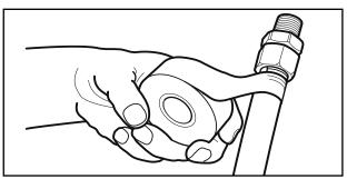
Figure: 4-5 Wrapping with self bonding silicone tape - begin on jacket.
