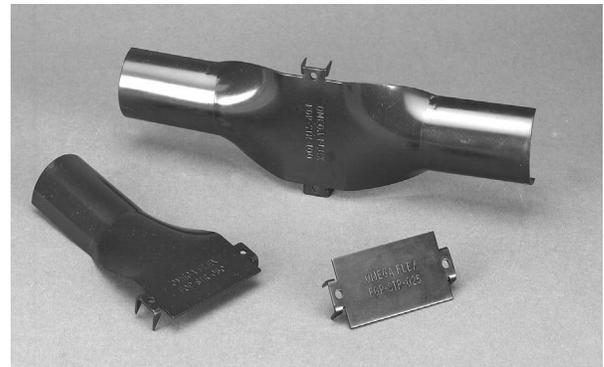
There are five striker plate configurations made from stamped steel and specially hardened to resist penetration from screws and pneumatic nail guns. These are quarter-striker, half striker, three quarter striker, full-striker and 6 inch X 17 inch flat plate striker. Spiral wound galvanized steel “floppy” conduit is available for use as additional protection.
