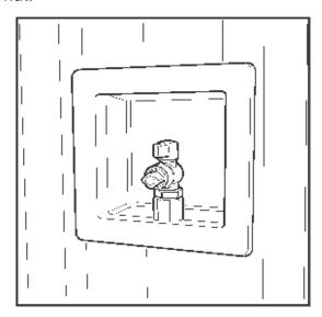
Install box cover after completion of drywall. If the gap between the edges of the box and the drywall is less than 1/4", no fire caulking is required.
