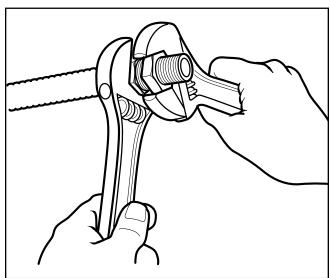
5. FINAL TORQUE: Tighten nut and adapter to the torque values shown in Table 4-4. For field installations use the following method: Tighten nut and adapter as though you were making up a flared tubing joint. Note relation between hex flats at this point and continue to tighten for two additional hex flats (one-third turn) to obtain required torque and final leak-tight seal.
