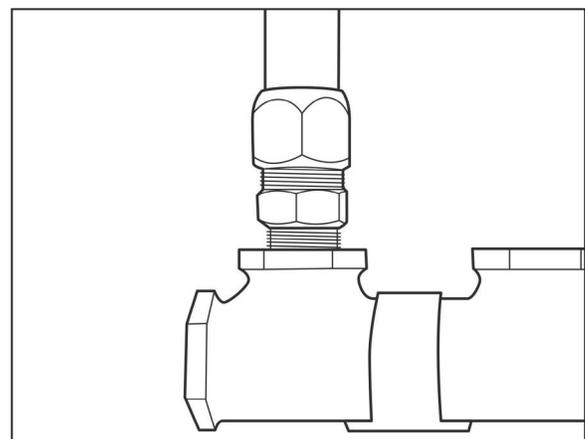
**DO NOT USE THREAD SEALANTS WITHIN THE FITTING. USE THREAD SEALANTS ONLY ON THE NPT THREADS**
