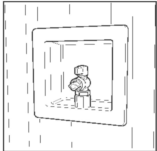
8. Install box cover after completion of dry-wall. If the gap between the edges of the box and the drywall is less than 1/4", no fire caulking is required.
