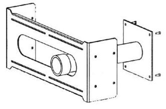
Stud Bracket (Mount between two studs.)
