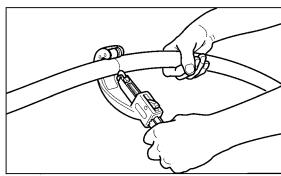
Unreel pipe into trench or on the ground and cut to desired length plus one additional foot. Cutting up to 1" size can be done with a large tubing cutter. For 1-1/4 to 2 inch sizes, a reciprocating saw is recommended.
