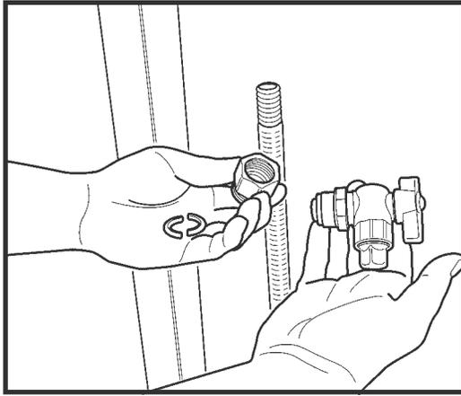
3. Disassemble nut and split rings from valve.
