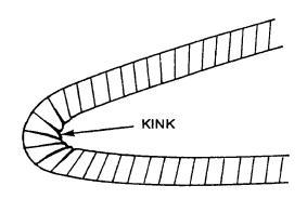
Figure: 5-3 – Repair Necessary.
