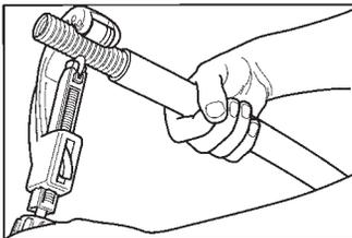
pipe to strip length specified in Table: 4-8. Cut slowly in the root of the corrugation in the same manner you would cut copper tubing. Inspect end of pipe for a clean cut without tears in corrugation.
