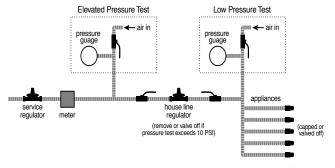
Figure: 6-1 – Pressure Test Requirement for a 2 PSI System
