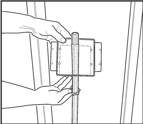
2. Remove box cover and slip locknut and box over end of pipe.
