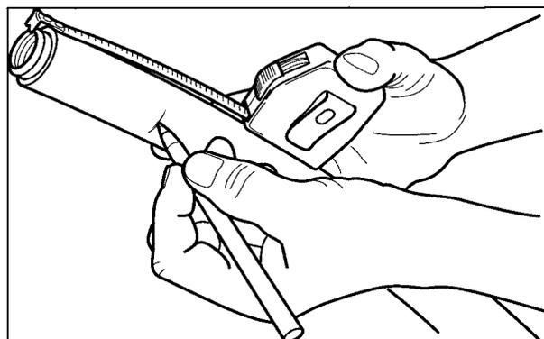
2. Mark the sleeve at specified length on the Strip Length Chart (Table: 4-8) - plus 2 inch.
