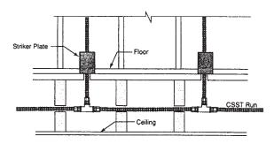
Figure: 4-4 Multiple outlets along main tubing run
