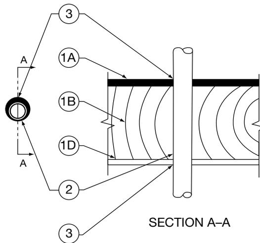
1. **Floor Assembly** - The 1 or 2 hr fire-rated wood joist, wood truss or combination wood and steel truss Floor-Ceiling assembly shall be constructed of the materials and in the manner described in the individual L500 Series Design in the UL Fire Resistance Directory. **The F Rating of the firestop system is equal to the rating of the floor-ceiling and wall assemblies.** The general construction features of the floor-ceiling assembly are summarized below:
