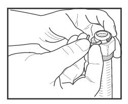
4. Slip nut over end of pipe and insert split rings into valley of the first corrugation.
