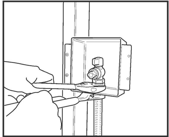
6. Slide box up and over the threads on the bottom of the nut and mount box firmly to stud. **Provide full support by fastening both mounting tabs to structure where required by local codes.**
