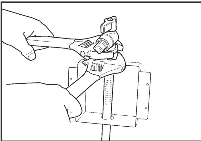
5. Thread 90 degree ball valve onto nut and tighten so valve outlet faces forward. It is recommended that crescent wrenches be used to avoid damaging valve or nut. **Do not use thread sealants on this connection.**
