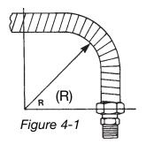
1. Multiple tight bends can restrict the gas flow and increase pressure drop. The tightest bend allowed for each size of **CounterStrike®** is shown in Table: 4-1.
