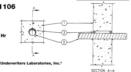
**1. Wall Assembly-** Min 4-7/8 in. or 6-1/8 in. thick lightweight or normal weight (100-150 pcf) concrete for 1 or 2 hr rated assemblies, respectively. Wall may also be constructed of any UL Classified **Concrete Blocks\***. Max diam of opening is 3-1/2 in.
