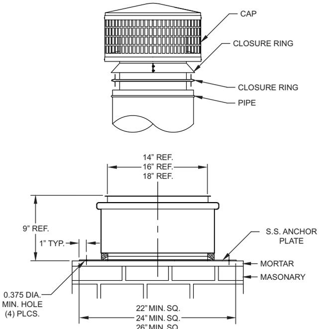
FIG. 15b 14TG, 16TG, AND 18TG ANCHOR PLATE
