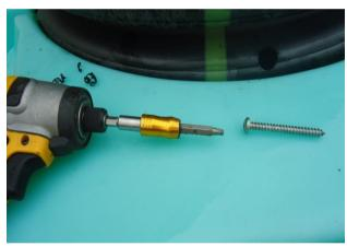
6. Drive screws in at approximately 45 degree angle, starting at the end toward the center of the tank.
