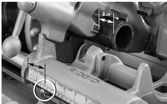
Figure 20B – Length Gauge Pointer At Desired Length
