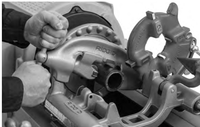
Figure 21 – Cutting Pipe with Cutter
