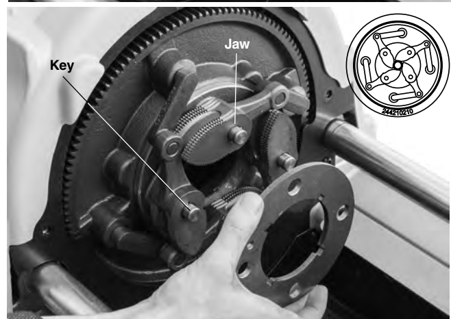
Figure 32 – Changing Auto Chuck Machine Jaws
