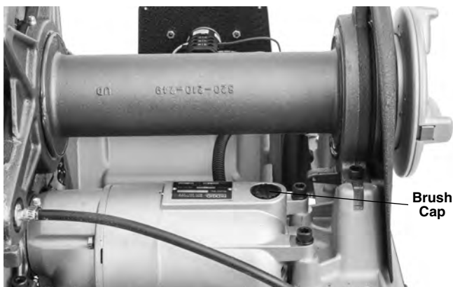
Figure 34 – Removing Motor Cover/Changing Brushes
