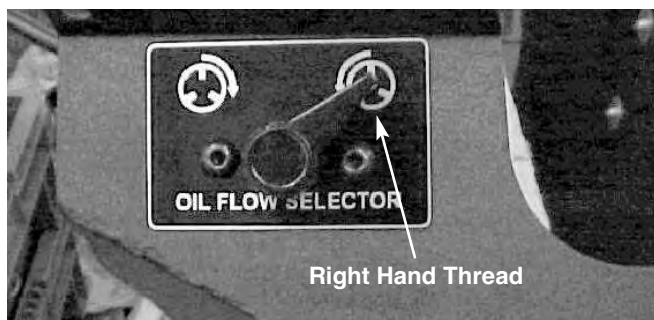
Figure 24 – LH or RH Oil Flow Selector
