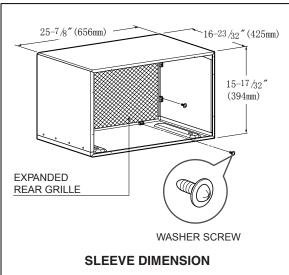
•If any portion of the sleeve"s exterior is exposed to the interior room side it is recommended to field insulate all exposed areas prior to installing chassis to avoid condensation from forming on exposed areas.
