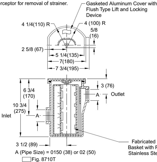
**NOTE:** Allow 14 1/2" (370) above interceptor for removal of strainer.
