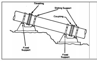
Support for all sizes of pipe in length to 40 ft. (12m). Suitable for any pressure. For any terrain including steep grades (hillsides). Pipe must be tied to only one support.
