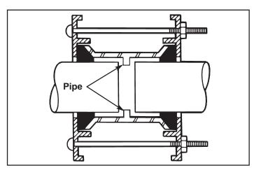
Pipe stops consists of a restriction in the center of the coupling sleeve to prevent the pipe from passing through the sleeve, and are available in most couplings upon request.
