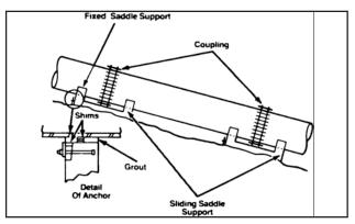
Support for all sizes of pipe in lengths to 40 ft. (12m). Suitable for any pressure. For any terrain including steep grades (hillsides). Pipe must be tied to only one support.
