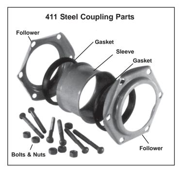
Smith-Blair water couplings consists of one cylindrical sleeve with conical inner surfaces at each end; two resilient, wedge shaped, specially-compounded rubber gaskets; two ring shaped followers; and a set of high-strength, low-alloy track head, oval neck, rolled-thread bolts with heavy hex nuts.
