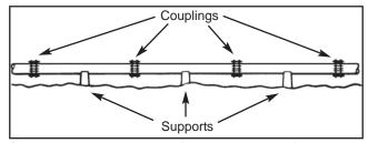
Support for 6 to 16 inch (150m to 400mm) diameter pipe in length to 20 ft. (6m) at pressures not to exceed 25 psi (1.7 Bar). Pipe to be tied to each support.
