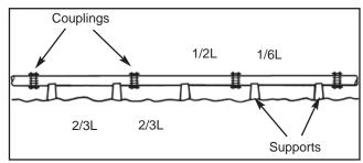
Support for pipes any size in length to 40 ft. (12m) Suitable for any pressure. Each length to be tied to one support to allow for expansion/contraction and isolate movement to each length of pipe. For use only where terrain is relatively level.
