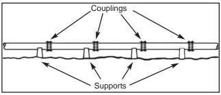
Support for 6 inch (150mm) and smaller diameter pipe in pipe length up to 20 ft. (6m) suitable for any pressure. Pipe must be tied to each support to accommodate high pressures and to isolate the pipe movement resulting from expansion/contraction in each length of pipe.
