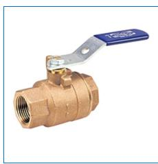
**Specifications UPC** Code 039923675347 Type Ball Valve T -- Female NPT Thread (FIPT) **Connection Type** Valve Size 3 Material Bronze CS Standard Lever Handle **Valve Operator** T58070 3 THRD BALL CONV PT BRZ **Description** eClass Classification Bronze Ball Valves All Type of Item Valve **Valve Pressure Rating (SWP)** 150 PSI / 10.3 Bar SWP **Turns/Operation** Quarter-Turn
