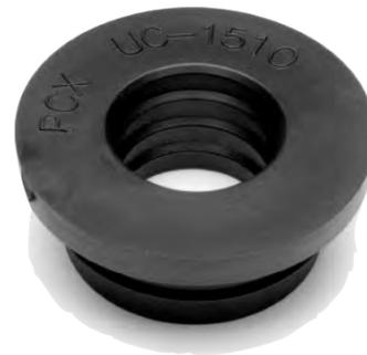
Use PIPECONX utility connectors to connect 1" or 3/4" CPVC and copper pipe to 1-1/2" DWV Schedule 40 plastic sockets (ABS or PVC) with a simple press fit. Our utility connectors are not for use in pressure water systems unless appropriate solvent cement is applied to the fitting socket and the utility connector.
