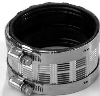
PIPECONX shielded couplings are elastomeric sleeves with stainless steel shields for use in joining cast iron, plastic, steel, copper and tubular in sewer and DWV systems.
