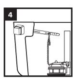
Connect flapper to arm hole. Chain needs slight slack (small J shape) when flapper is in closed position. Test for proper flush and adjust slack if needed. Tighten locknut by hand. DO NOT overtighten as it may crack tank.
