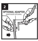
Unthread nut from new push button model. Remove nut, adapter and lever arm. Slide push button shank through tank hole (flat groove on threads facing up). Slip lever arm back onto shank. If does not fit snugly, slide adapter on (flat side facing button) then lever arm.
