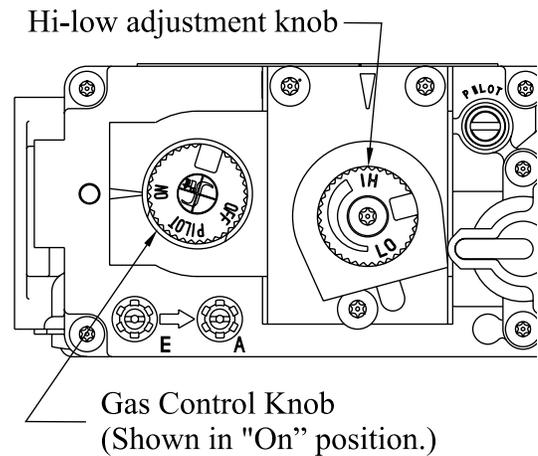
Figure 24. 'Hi-Lo' Adjustment on the M40DV-ST's gas valve.
