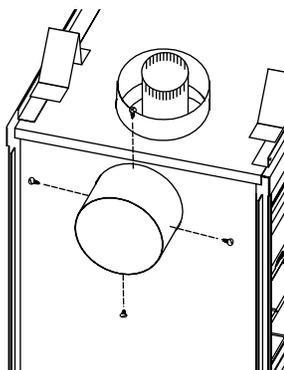
Figure 5c. Flue cover installation for top vented fireplace.
