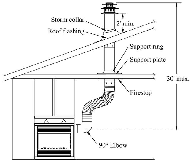
Figure 11a. Vertical venting with 1 offset (1 offset=two 90° bends).
