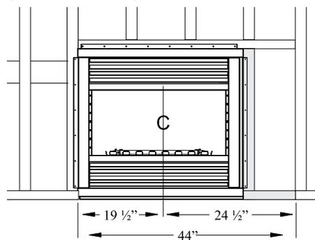
Figure 2b. Back-framing to finish enclosing the fireplaces can be constructed on either the left or right side.
