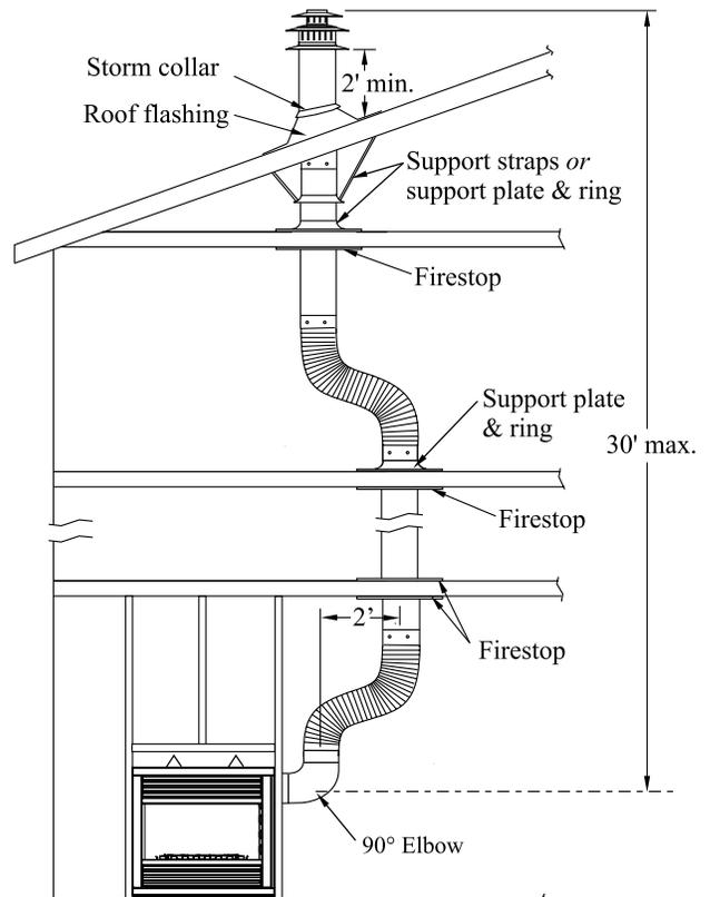
Figure 11b. Vertical venting with 2 offsets (1 offset=two 90° bends).
