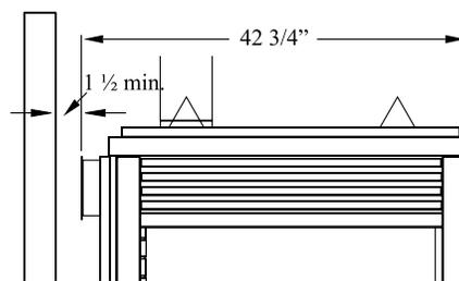
Figure 2c. Flue cover clearances to combustibles when installing the unit in a top vent configuration.
