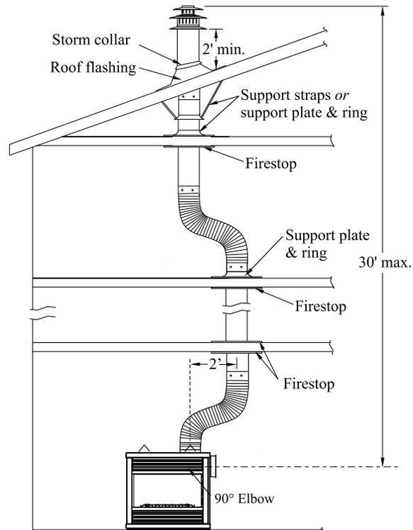
Figure 18. Vertical venting using 2 offsets (1 offset= two 90° bends).
