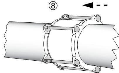
**Step 9** • Tighten bolts such that the end ring flanges remain parallel and the gaskets are evenly compressed. Bolt tightening should be done evenly, alternating to diametrically opposite positions at approximately 20 ft-lbs increments. Tighten to 75 - 90 ft-lbs.
