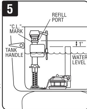
When installed the top of the overflow pipe of the flush valve must be at least 3" below the top of the fill valve.
