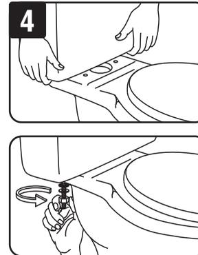
Before replacing the tank on the bowl, place metal washer and hex nut onto bolt under tank and hand tighten hex nut. Then place tank back on the bowl gasket so that tank to bowl gasket fits evenly. Level tank. Under the bowl attach rubber washer, metal washer and metal hex nut. Tighten the hex nuts under the bowl evenly until the tank is stable and doesn't rock. **DO NOT OVERTIGHTEN** or the tank or bowl could break.
