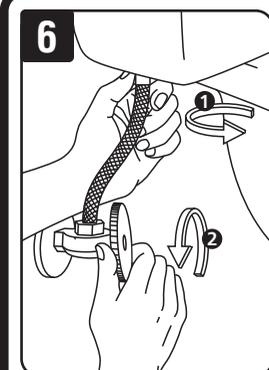
Reconnect water supply line to bottom of fill valve (1). Turn on water supply and check for any leaking. If leaking, turn nut just enough to stop leaking. Then flush toilet to check.
