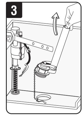
Remove tank-to-bowl gasket and large nut from old flush valve. Then remove flush valve from tank.
