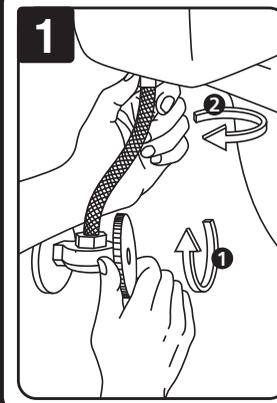
Turn off water supply (1). Flush toilet and remove excess water from tank with sponge. (2) Place bucket or towel under water supply line and remove nut of water supply line from bottom of toilet fill valve.
