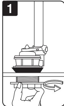
Place flush valve in tank. Position the overflow pipe toward the back of the tank. Do not cover bolt holes. Hand tighten flush valve lock nut. **DO NOT OVERTIGHTEN** or tank may crack.
