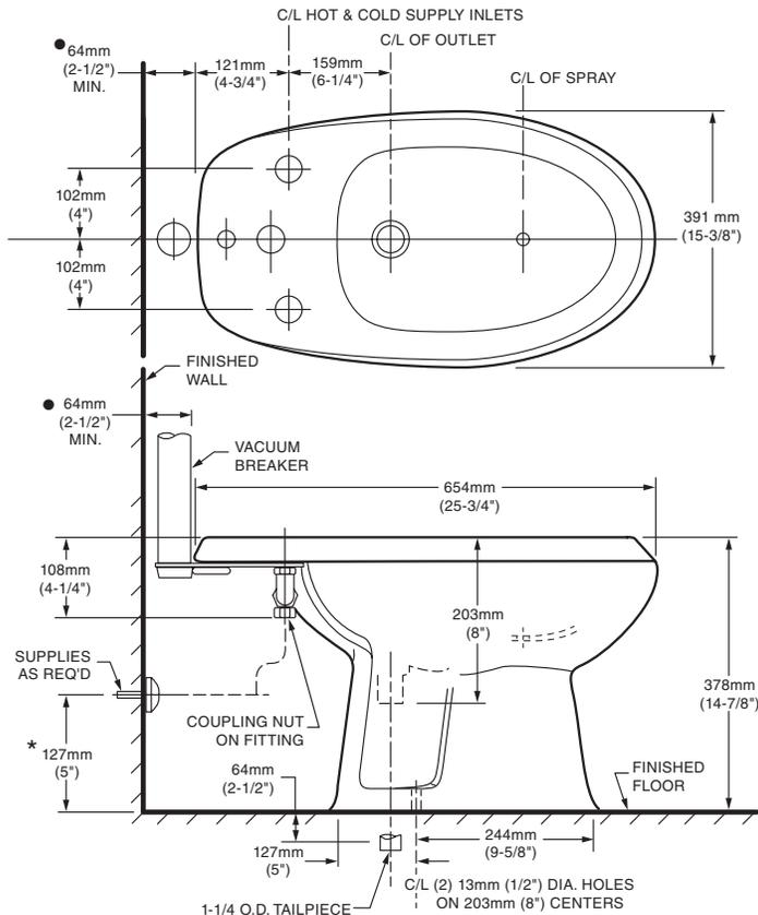
**1** The bidet is not furnished with a trap. Provisions must be made for the installation of a trap in the floor.
