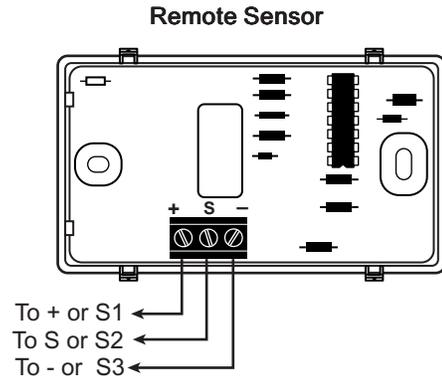
**Figure 3 – Single Stage (1F97-1277) Touchscreen Thermostat Indoor/Outdoor Remote Sensor Wiring (F145-1328/F145-1378)**
