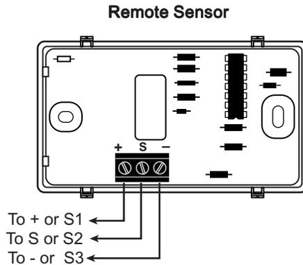
**Figure 4 – Staging Multi-Stage or Heat Pump Touchscreen Thermostat (1F95-1277) Indoor/Outdoor Remote Sensor Wiring (F145-1328/F145-1378)**
