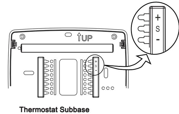
**Note:** When using shielded cable, connect shield of 18 or 20 gauge 3 conductor cable to - or S3 on thermostat subbase.
