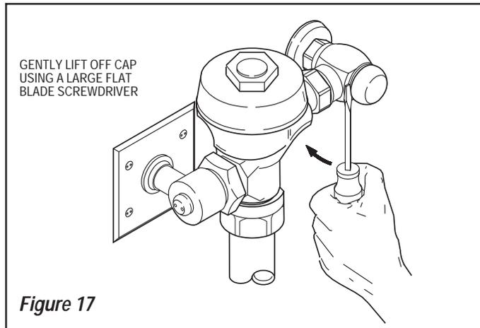
**Important:** DO NOT install the Cap onto the Sleeve unless the Sleeve has been threaded onto the Control Stop Bonnet. If assembled when off of the Control Stop, the Sleeve WILL NOT come apart from the Cap.
