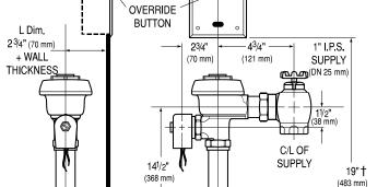
Position of Sensor Box can be raised or lowered 1" (25 mm) if in conflict with Handicap Grab Bars.
