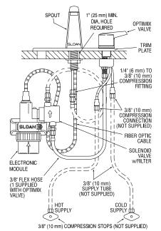
EBF-187 Faucet with BDM and BDT Variation Mixing Valves for Hot and Cold Water Supply (shown with 4" trim plate)
