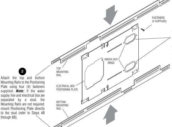
When Installing The Positioning Plate Over a 1 Inch Copper Supply Pipe ONLY — Remove the appropriate Knock-out ring by inserting a screwdriver through the opening and lightly twisting the ring to snap it out.
