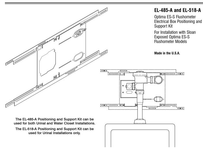
This manual only covers installation of the Optima ES-S Flushometer Electrical Box Positioning and Support Kit. Use these instructions in conjunction with the separate installation instructions included with each ES-S Flushometer.
