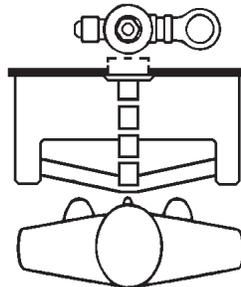
3. When the user steps away from the OPTIMA Sensor, the loss of reflected light initiates an electrical "one-time" signal that energizes the Solenoid Operator, and activates the Flushometer to flush the fixture. This occurs approximately three (3) seconds after indication. The circuit then automatically resets and is ready for the next user.
