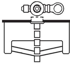
2. As the user enters the beam's effective range, 15 to 30 inches (381 mm to 762 mm), the beam is reflected into the OPTIMA'S scanning window and transformed into a low voltage electrical signal that activates a ten-second time delay circuit. The time delay circuit eliminates false operation from passers-by in the rest room. Once the time delay is completed, the output circuit is alerted and continues in a "hold" mode for as long as the user remains within the effective range of the sensor.
