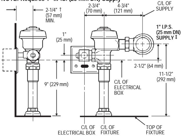
† IF THIS DISTANCE IS GREATER THAN 3" (76 mm) AN EL-226 EXTENSION ADAPTER IS REQUIRED. SPECIFY ONE EL-226 FOR EVERY 1-1/4" (32 mm) INCREMENT OVER 3" (76 mm).
