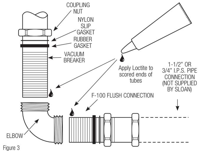
Loctite can also be used to secure Push Button Flange. See Sealant package for details.
