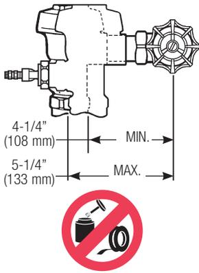
Maximum adjustment of Sloan Adjustable Tailpiece is 1/2" (13 mm) IN or OUT from the standard 4-3/4" (121 mm) (centerline of Flushometer to centerline of Control Stop). If rough-in measurement exceeds 5-1/4" (133 mm), consult factory for longer tailpiece.
