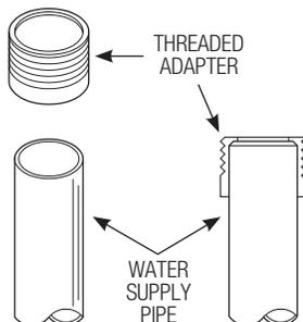
**B** Install the Sloan Bak-Chek® Control Stop to the water supply line with the outlet positioned as required.
