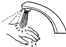
3. When hands are removed, the water flow automatically stops. The faucet is then ready for the next user.
