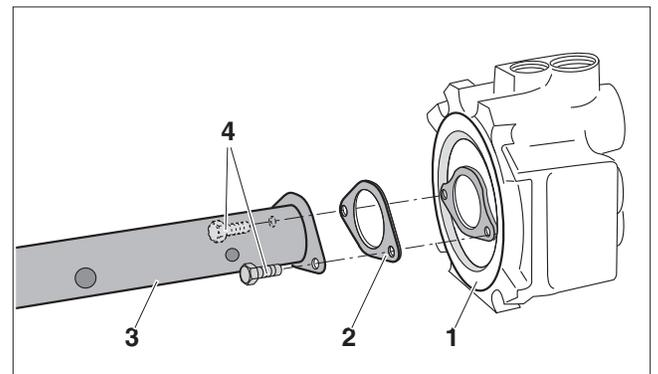
Fig. 18 Fitting feed pipe on supply/return header
