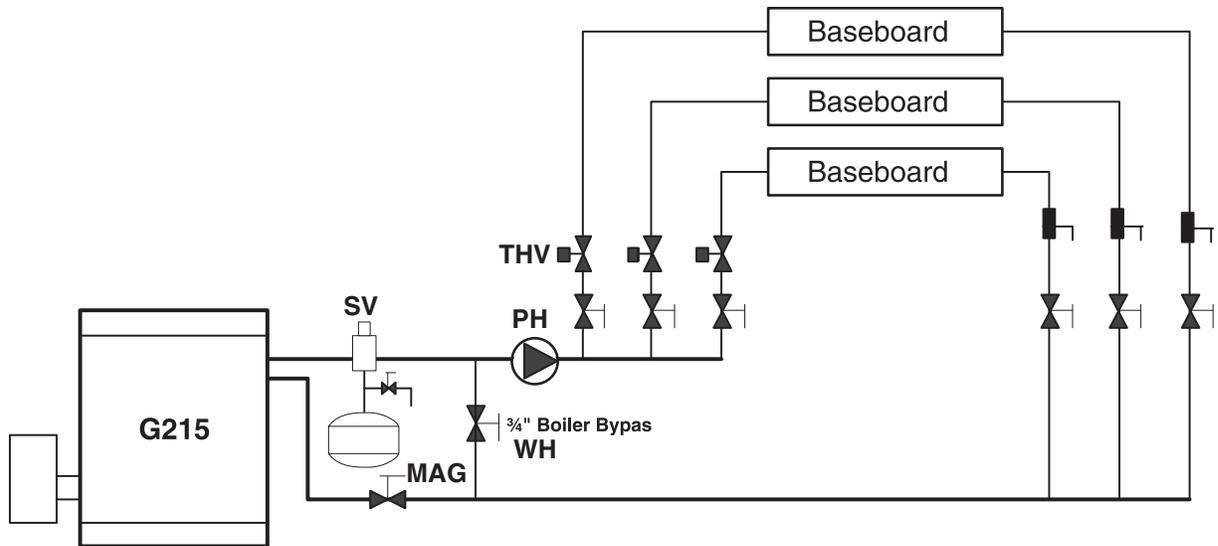
Fig. 74 Multiple circuits of water diversion for systems with a high water volume
