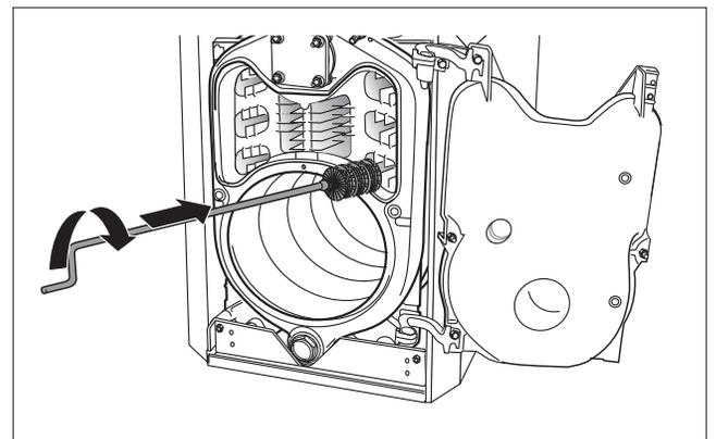
Fig. 68 Brushing out the flue gas passages
