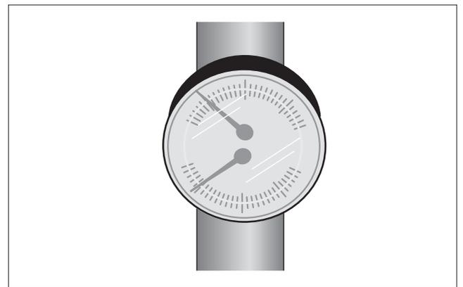
Fig. 50 Pressure/temperature gauge
