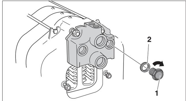
Fig. 21 Seal connections that are not required.
