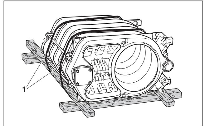
Fig. 27 Boiler block on pallet (as delivered)
