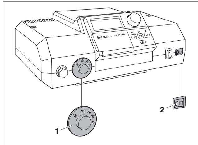
Fig. 59 Switching on the control (for example Logamatic 2000)
