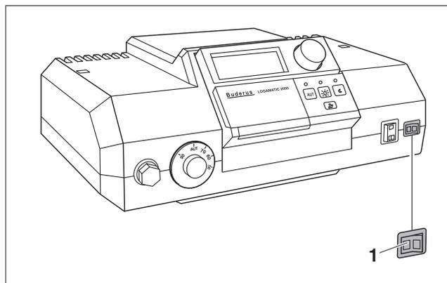
Fig. 65 Shutting down the heating system (Logamatic 2000)
