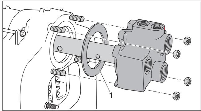
Fig. 19 Fitting feed pipe and supply/return header
