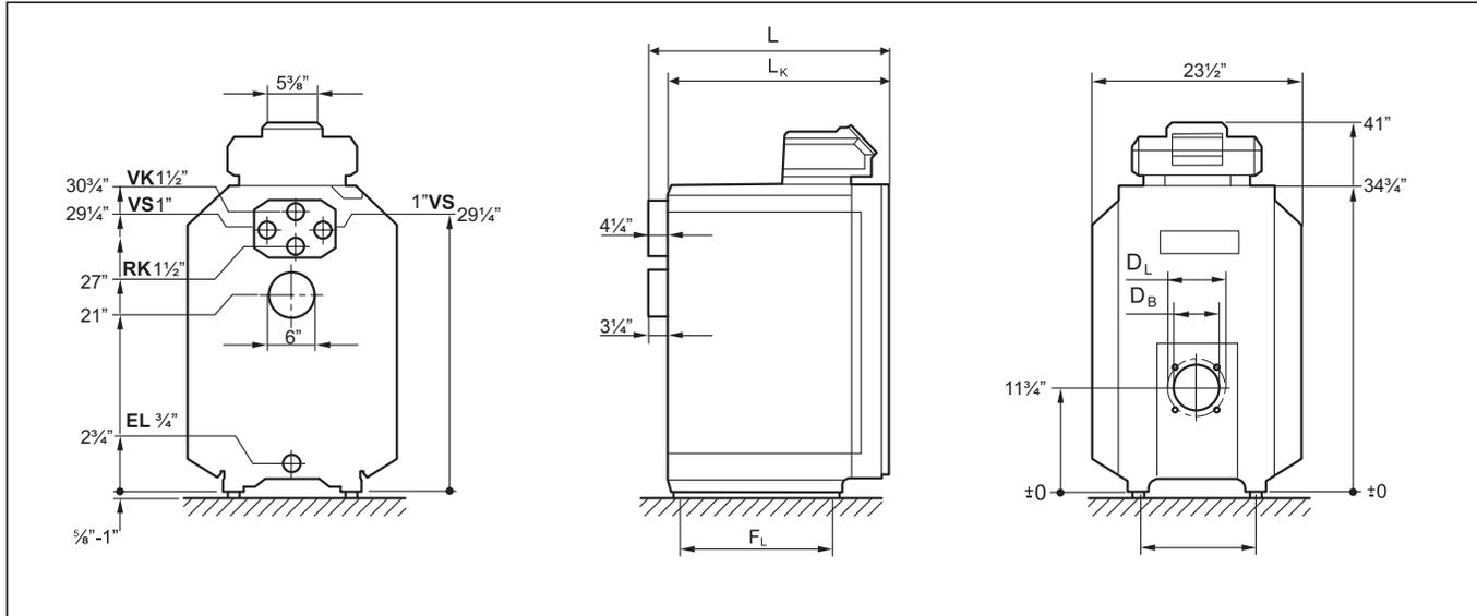
Fig. 2 Connections and dimensions (measurements in inches)
