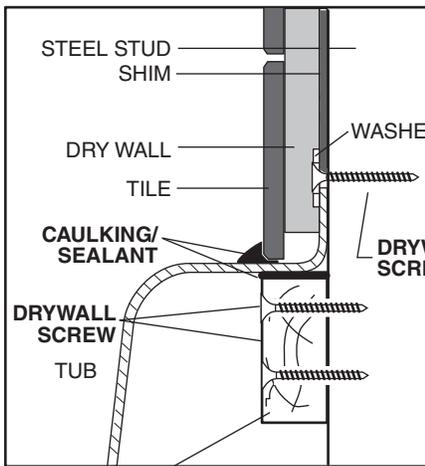
FOR STEEL STUDS SUPPORT THE WOOD 2 X 4 STRINGER TO THE FLOOR IN 3 PLACES
