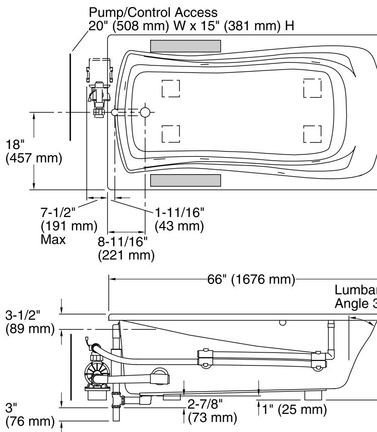
No change in measurements if connected with drain illustrated. (K-7161-AF)
